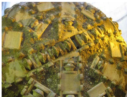
Fig. 5. Worn cutter-disc after tunneling in cobble and gravelly soil.
