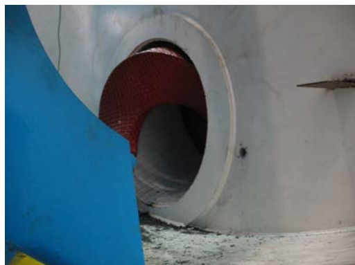
Fig. 4. Ribbon-type screw conveyor to transport cobble particles.
